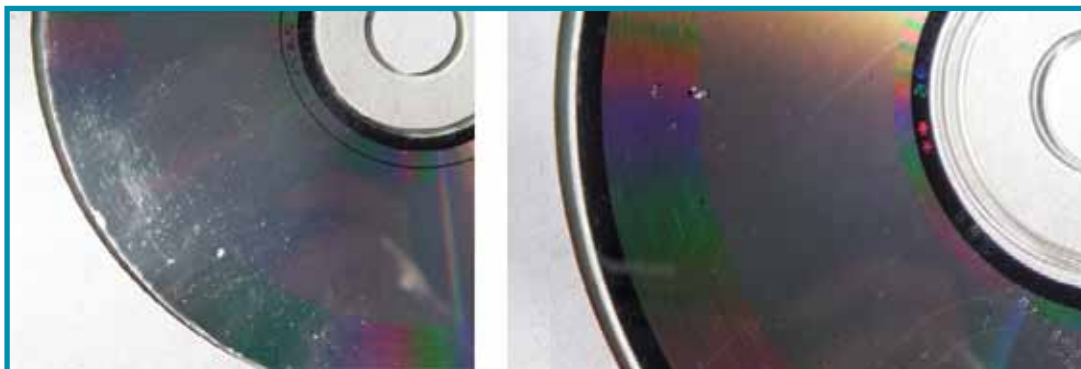
Photo 3: Sample pressed music CDs showing pin holes in aluminium reflective layer affecting data/tracks. (David Sylvian, 1987 CDV 2471 and Betty Blue, 1986 CDV 2396).
